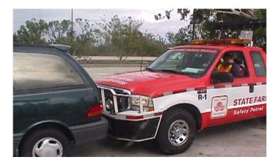
Figure 11 – Push Bumper Relocation
