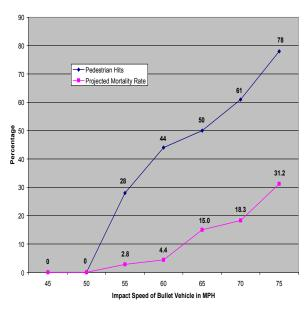
When the condition of the roadway was modified to represent slippery/snow-covered pavement, the in-line configuration without a barrier resulted in approximately 36% misses, 6% near misses, and 58% hits. On those occasions when the pedestrian officer was struck, the average impact speed ranged from 12 to 31 mph and the projected mortality ranged from 4.8 to 30.4 percent. The following graph illustrates the relative effectiveness of the configuration.
