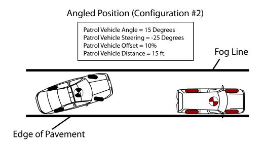
and right-side officer approaches are analyzed. The diagrams illustrate the vehicle positioning configurations used in the analysis.
