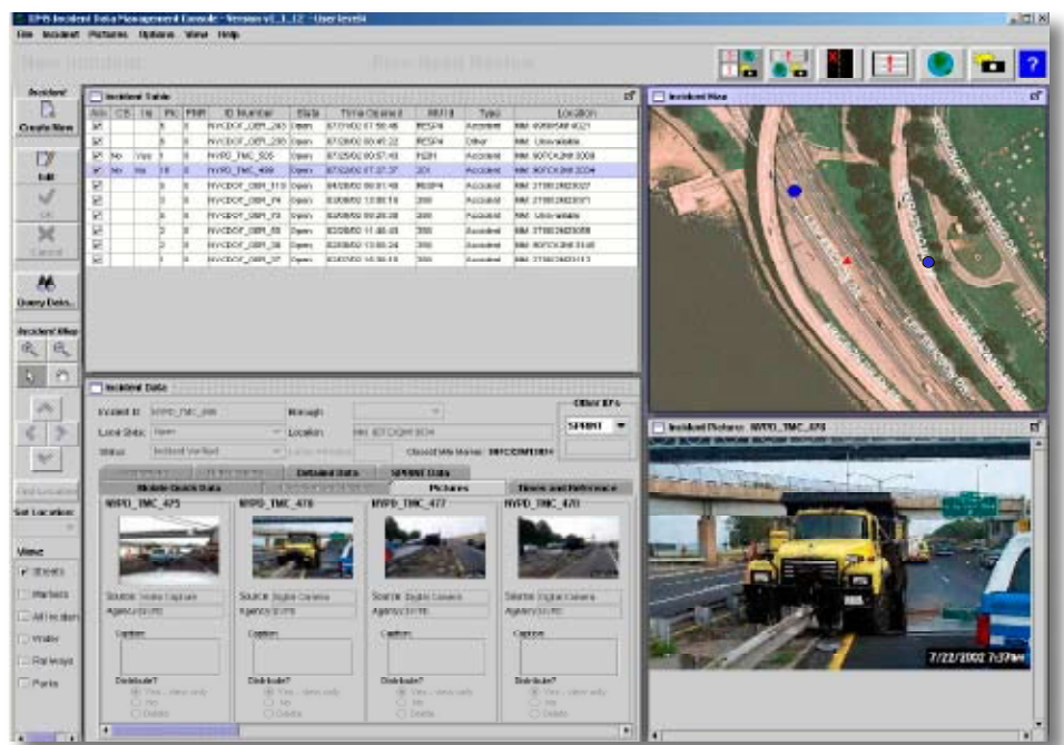
Screenshot from New York City's Integrated Incident Management System (IIMS), which enables NYPD officers to transmit incident scene photos to NYCDOT's Traffic Management Center, speeding prompt dispatch of appropriate responder resources.
